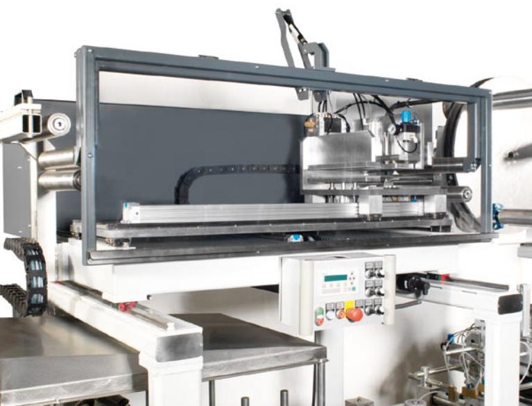
The automatic cross-cut and jointing unit allows a continuous production even in case of film change.
