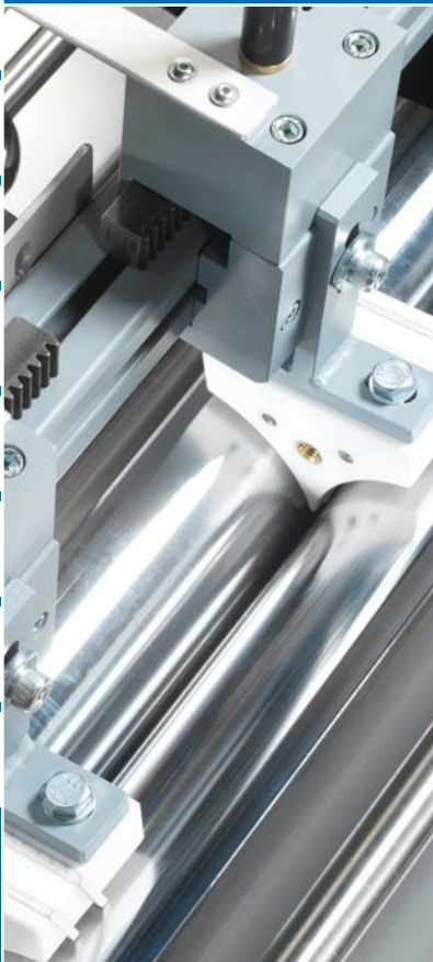
Glue quantity and application width are exactly defined through gap and scraper.
