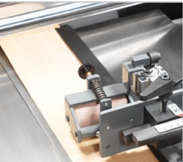
A pneumatically regulable controller cylinder ensures an exact guide of the veneer roll in the infeed table.
