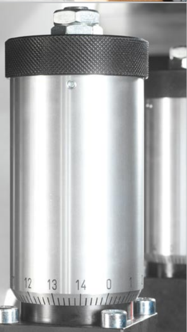
The pressure cylinders in the calender station allow being adjusted precisely and individually in 0,02 mm steps.
